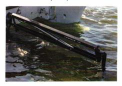
Lewmar shallow water anchors do not require hydraulic pumps or hoses, making them low-maintenance and easily installed
