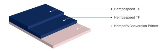
For full season protection - no need to remove old coating, just 1 coat of Hempel's Conversion Primer needs to be applied before applying 2 coats of Hempaspeed TF.
