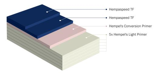
For a full season protection, the substrate needs to be sealed with Hempel's Light Primer  $(300\mu m\ dft)$  before applying Hempel's Conversion Primer and 2 coats of Hempaspeed TF. Follow stated overcoating intervals between the primer and product to ensure intercoat adhesion.
