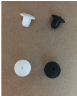
LAVAC: TLZ9251 Bleed plug kit for inlet hose 2 sizes of plug with hole that allows air into system preventing siphoning and releasing vacuum when pumping stops. Size of hole determines how much water remains in bowl.
