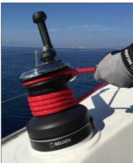
The grip on the drum and the ingenious self-tailer allow you to let the winch handle remain in the winch while pulling the slack. Check out the video.
