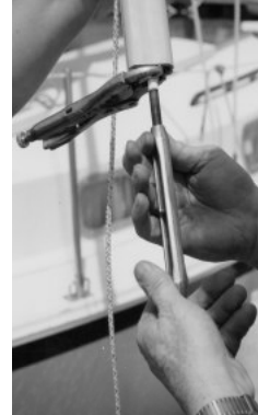
screwing turnbuckle on stud
