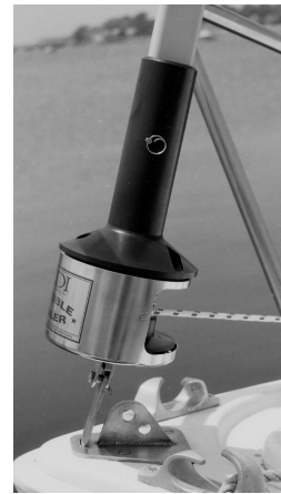
Furler w/ luff support pin installed
