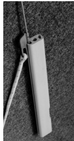
Inserting FF6 traveler into top of luff
