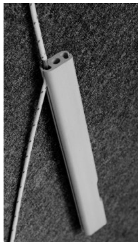
Inserting FF4 ferrule into top of luff
