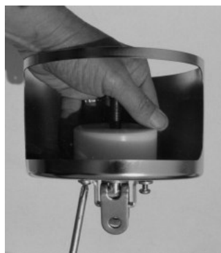
Assembling cup, bearing and antirotation strap
