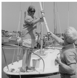
pushing extrusion up forestay
