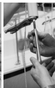
screwing turnbuckle on stud
